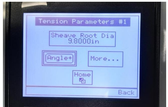
The “Angle +/-” setting just changes which direction of sheave movements is interpreted as a positive angle by the inclinometer installed in the sheave assembly.
