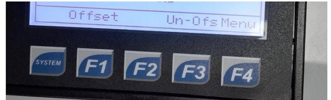
The F3 "Un-Ofs" button can undo the zeroing to instead display the absolute amount of cable paid out.
