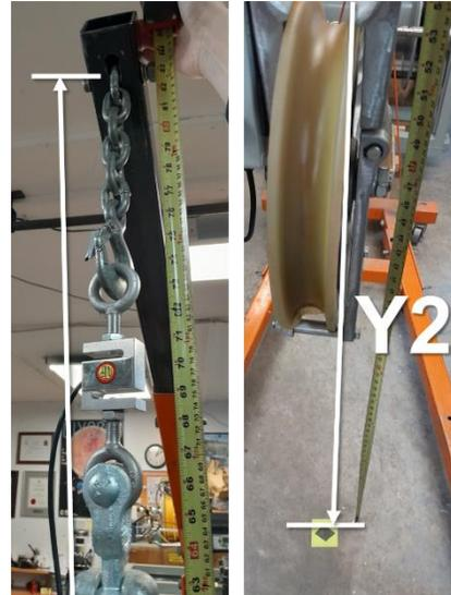
💡 If it is not possible to safely measure X2 and Y2 in the A-frame's deployment position, use the A-frame's length and deployment angle to help calculate X2 and Y2.
