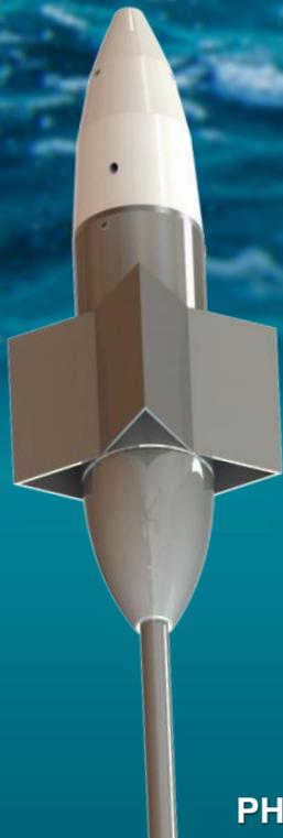
The **STING MkII** is a portable, tethered free-falling penetrometer (FFP) for measuring seafloor bearing strength. It is simple to operate such that first-time users can perform a seafloor analysis on sediments ranging from very soft mud to medium-density sand with minimal instruction.
