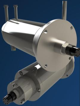
A.G.O. Environmental's AGO-SR08 and AGO-SR08B slip ring units are designed to enclose affordable basic slip ring modules in a sealed, stainless steel housing to protect them from the elements in outdoor and marine applications. They are principally designed for installation on A.G.O.'s winches, but can also be purchased for installation on other winches or equipement.
