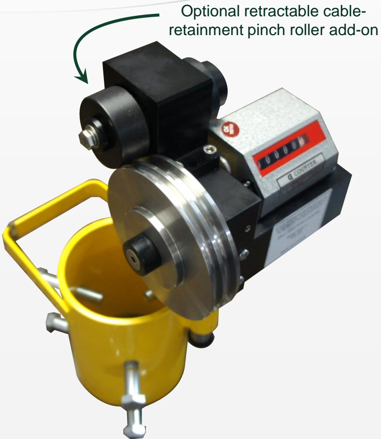
Wheel centered over drill-collar mount for operation.
